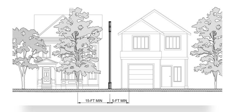
Type 4 Poles Shall be Placed on or in line with property lines separating adjoining lots
